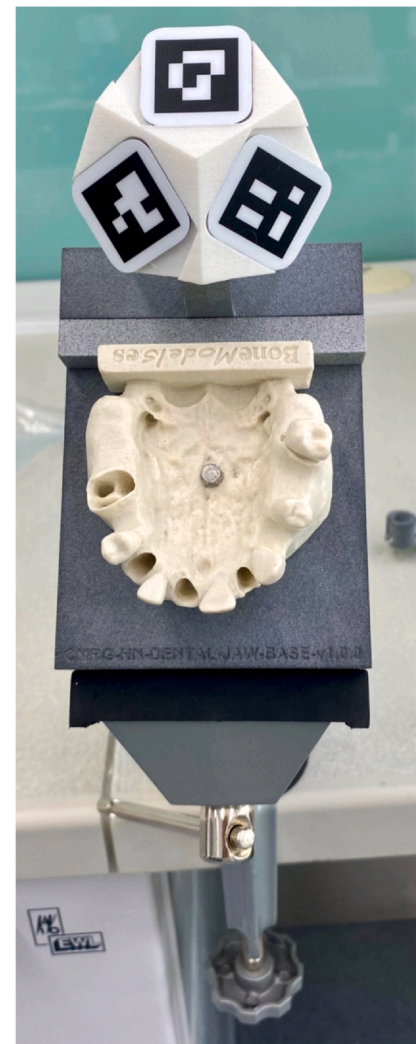
Fig. 4. Fixation technique of the jaw model with custom-made pointing device for registration.
