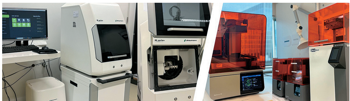
Figure 2.—Digital manufacturing methods in dentistry: CAD/CAM subtractive milling process, and additive 3D printing technology. The images depict representative equipment used in each method.
