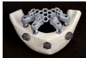
Figure 5. Reference model with splinted scan bodies and OptiSplint device.
