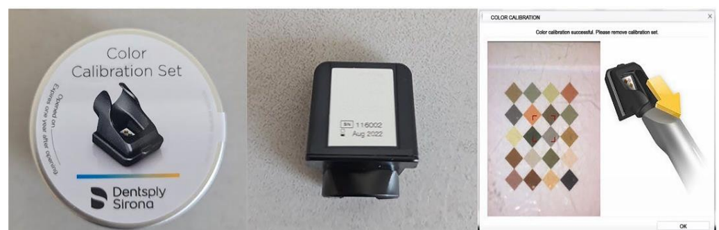
Figure 3. Cerec Omnicam color calibration set—required to successfully perform the calibration step before shade analysis.
