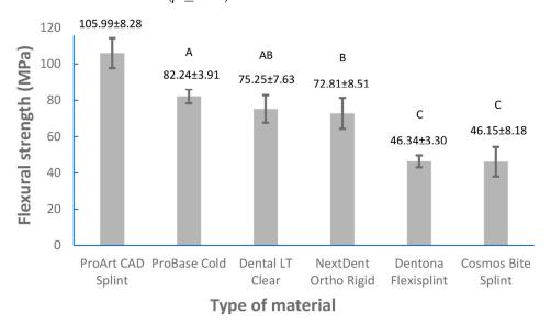
**Figure 2.** Mean values ( $\pm$ SD) of flexural strength for the tested groups. Identical uppercase letters above a column indicates that there is no significant difference between the tested groups (Tukey post-hoc test (p > 0.05)).
