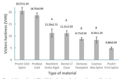
**Figure 3.** Mean values ( $\pm$ SD) of Vickers hardness for the tested groups. Identical uppercase letters above a column indicate that there is no significant difference between the tested groups (Tukey post-hoc test (p > 0.05)). VHN, Vickers hardness number.
