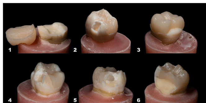
Fig. 5. Representative examples of failure modes after load to failure test: 1) Dislodgement of the restoration; 2) Fracture of enamel and dentin; 3) Fracture of the restoration; 4) Fracture of the restoration and enamel; 5) Fracture of the restoration, enamel, and dentin; 6) Root fracture.
