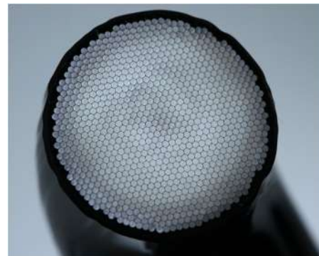
FIGURE 4 Construction of a LCU optic tip containing a glass-fibre bundle (Bluephase PowerCure, Ivoclar AG).
