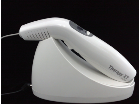
FIGURE 10: Laser unit used ( \lambda = 660 \text{ nm} ) and optical fiber (Therapy XT-DMC, São Carlos, SP, Brazil).
