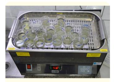
Figure 5: Implants under the first asepsis (ultrasonic tank).
