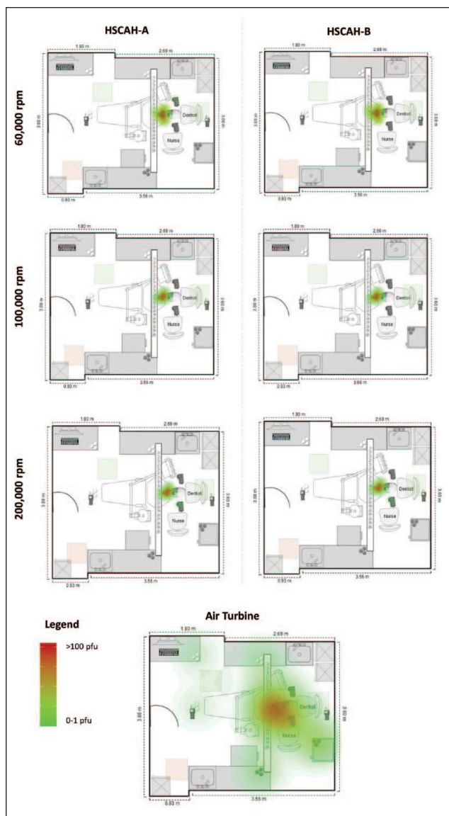
Figure 2. Heatmap representation of bacteriophage dispersal in the dental surgery, delineated by handpiece and cutting speed. Circles represent settle plate sampling points, gray (multiple time points) and white (single time point). Data from Vernon et al. (2021) for an air turbine are displayed as a comparator. Heatmaps were created using image overlay function of http://www.heatmapper.ca . pfu, plaque forming units.
